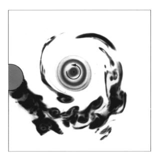
Fig. 5 LIF photograph in the horizontal plane *B* showing the sphere wake entrainment into the primary vortex core for a case with  $D/\sigma_0$ =4.3 and S/D=2
